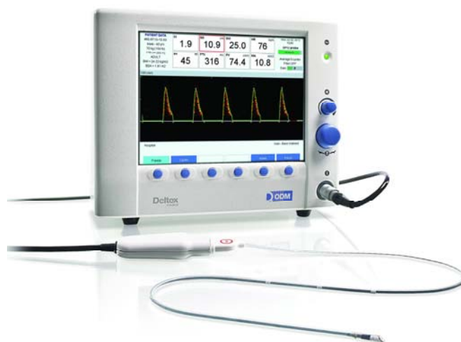
Figure 4. CardioQ-ODM™ Oesophageal Doppler Monitor.
